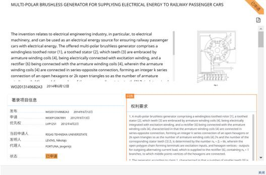
The screenshot shows a patent document viewer interface. The title is "MULTI-POLAR BRUSHLESS GENERATOR FOR SUPPLYING ELECTRICAL ENERGY TO RAILWAY PASSENGER CARS". The text describes an electrical energy source for railway passenger cars, mentioning a windingless toothed rotor, a toothed stator, and armature winding coils. A diagram of the generator is visible. Below the text, there is a table with patent information:
